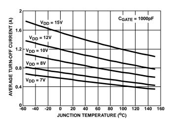
FIGURE 10. AVERAGE TURN-OFF CURRENT ( $V_{\mbox{\scriptsize DD}}$  TO 4V)
