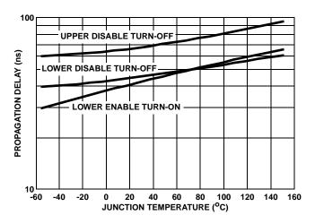
FIGURE 13. DISABLE PIN PROPAGATION DELAY
