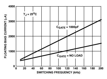
FIGURE 5. FLOATING  $I_{XHB}$  BIAS CURRENT
