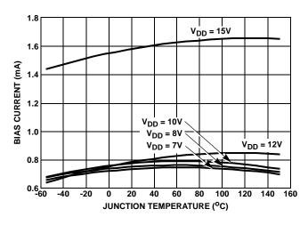
FIGURE 6. OFF-STATE I<sub>XHB</sub> BIAS CURRENT
