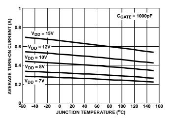
FIGURE 9. AVERAGE TURN-ON CURRENT (0 TO 5V)
