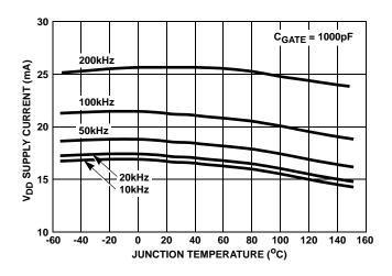
FIGURE 4. V<sub>DD</sub> SUPPLY CURRENT vs SWITCHING FREQUENCY
