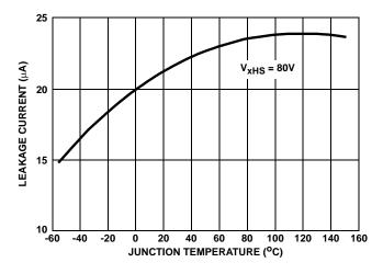
FIGURE 17. I<sub>xHS</sub> LEAKAGE CURRENT
