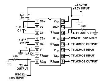
FIGURE 7. GENERAL TEST CIRCUIT
