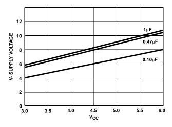
FIGURE 5. V- SUPPLY VOLTAGE vs V<sub>CC</sub>, VARYING CAPACITORS
