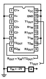
FIGURE 8. POWER-OFF SOURCE RESISTANCE CONFIGURATION
