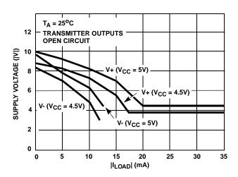
FIGURE 6. V+, V- OUTPUT VOLTAGE vs LOAD (HIN232)
