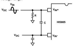
FIGURE 18. DC COUPLED SINGLE ENDED INPUT
