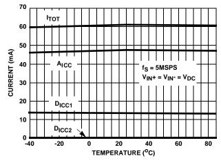
FIGURE 12. POWER SUPPLY CURRENT vs TEMPERATURE
