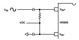
FIGURE 17. AC COUPLED SINGLE ENDED INPUT
