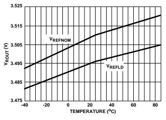
FIGURE 10. INTERNAL VOLTAGE REFERENCE OUTPUT (VROUT) vs TEMPERATURE AND LOAD
