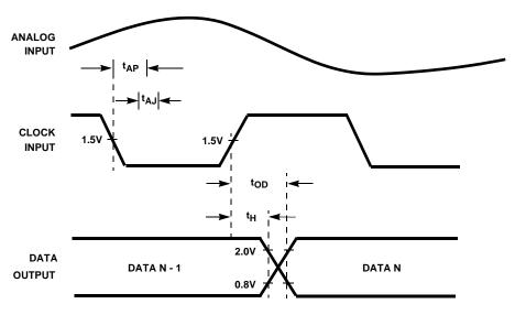
FIGURE 2. INPUT-TO-OUTPUT TIMING
