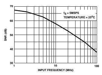
FIGURE 5. SIGNAL TO NOISE RATIO (SNR) vs INPUT FREQUENCY
