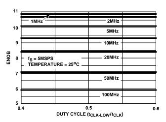
FIGURE 8. EFFECTIVE NUMBER OF BITS (ENOB) vs CLOCK DUTY CYCLE AND INPUT FREQUENCY
