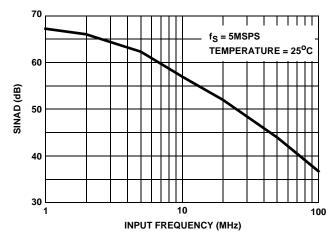
FIGURE 4. SIGNAL TO NOISE AND DISTORTION (SINAD) vs INPUT FREQUENCY
