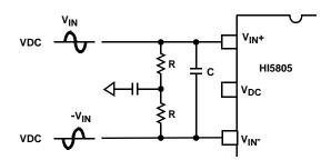
FIGURE 16. DC COUPLED DIFFERENTIAL INPUT
