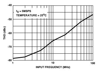
FIGURE 6. TOTAL HARMONIC DISTORTION (THD) vs INPUT FREQUENCY
