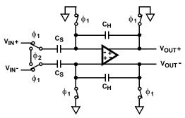
FIGURE 14. ANALOG INPUT SAMPLE-AND-HOLD
