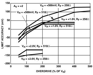
FIGURE 32. V<sub>H</sub> LIMIT ACCURACY vs OVERDRIVE
