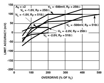
FIGURE 33. V<sub>L</sub> LIMIT ACCURACY vs OVERDRIVE
