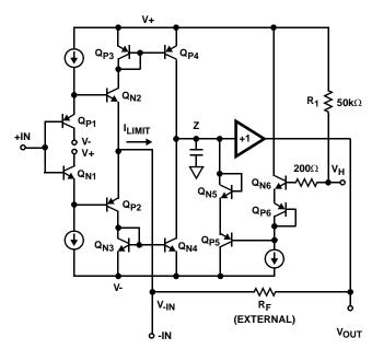
FIGURE 3. HFA1135 SIMPLIFIED VH LIMIT CIRCUITRY
