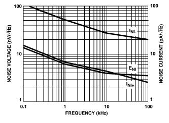
FIGURE 29. INPUT NOISE CHARACTERISTICS
