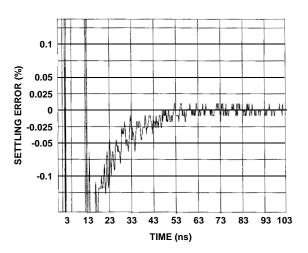
FIGURE 28. SETTLING TIME RESPONSE
