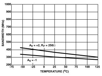
FIGURE 23. -3dB BANDWIDTH vs TEMPERATURE
