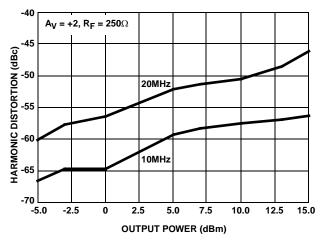
FIGURE 30. 2nd HARMONIC DISTORTION vs POUT
