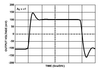
FIGURE 12. SMALL SIGNAL BIPOLAR PULSE RESPONSE
