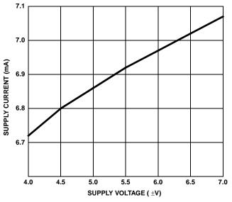
FIGURE 38. SUPPLY CURRENT vs SUPPLY VOLTAGE
