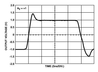
FIGURE 13. LARGE SIGNAL BIPOLAR PULSE RESPONSE
