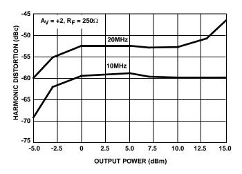
FIGURE 31. 3rd HARMONIC DISTORTION vs POUT
