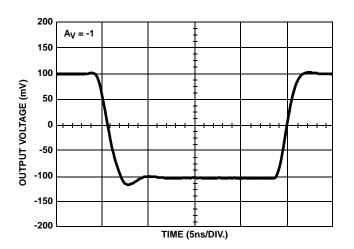
FIGURE 16. SMALL SIGNAL BIPOLAR PULSE RESPONSE
