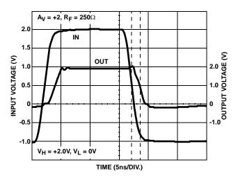
FIGURE 5. PULSE RESPONSE WITH LIMITING
