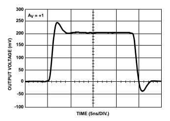
FIGURE 10. SMALL SIGNAL POSITIVE PULSE RESPONSE
