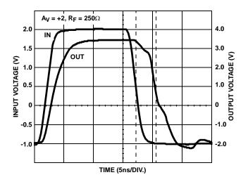
FIGURE 4. PULSE RESPONSE WITHOUT LIMITING
