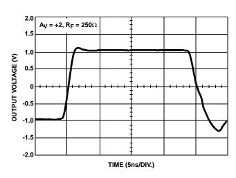
FIGURE 9. LARGE SIGNAL BIPOLAR PULSE RESPONSE
