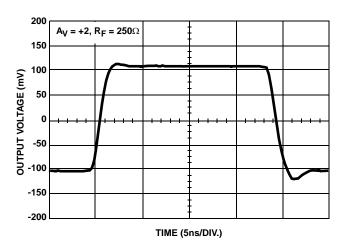
FIGURE 8. SMALL SIGNAL BIPOLAR PULSE RESPONSE
