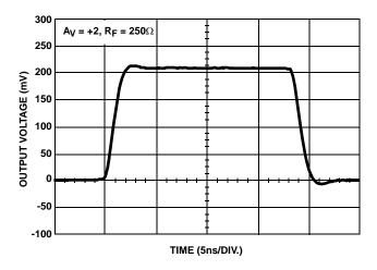
FIGURE 6. SMALL SIGNAL POSITIVE PULSE RESPONSE
