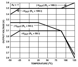
FIGURE 37. OUTPUT VOLTAGE vs TEMPERATURE
