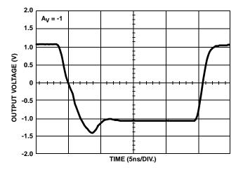
FIGURE 17. LARGE SIGNAL BIPOLAR PULSE RESPONSE
