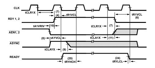
FIGURE 4. WAVEFORMS FOR READY SIGNALS (FOR SYNCHRONOUS DEVICES)
