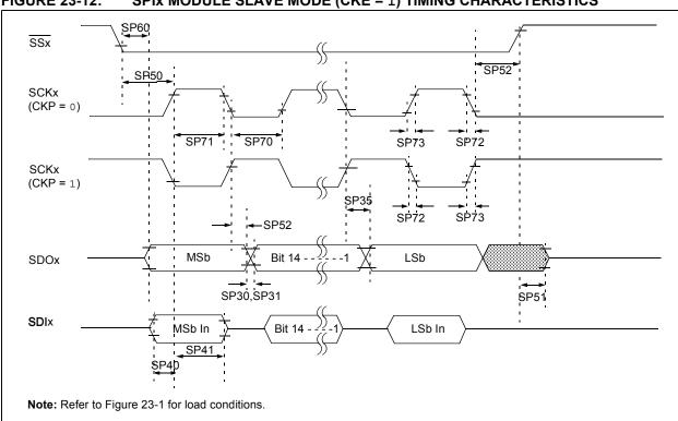
FIGURE 23-12: SPIX MODULE SLAVE MODE (CKE = 1) TIMING CHARACTERISTICS
