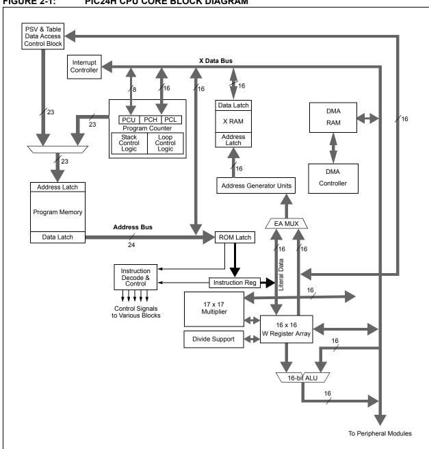
FIGURE 2-1: PIC24H CPU CORE BLOCK DIAGRAM
