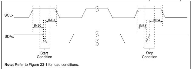
FIGURE 23-14: I2Cx BUS DATA TIMING CHARACTERISTICS (MASTER MODE)
