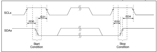
FIGURE 23-16: I2Cx BUS DATA TIMING CHARACTERISTICS (SLAVE MODE)
