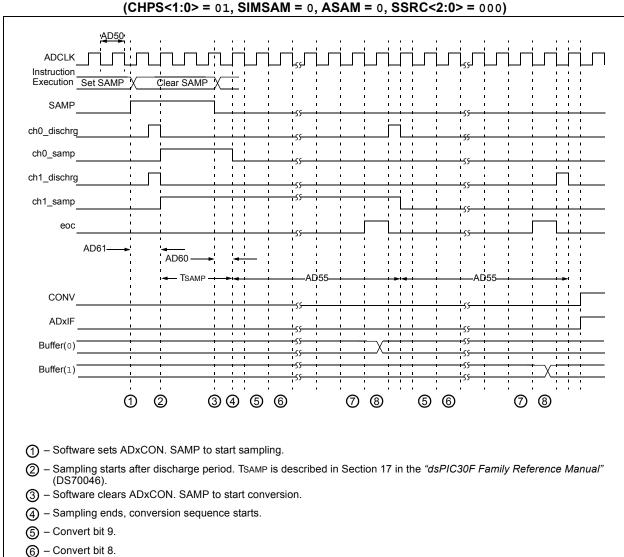
FIGURE 23-18: A/D CONVERSION (10-BIT MODE) TIMING CHARACTERISTICS (CHPS<1:0> = 01, SIMSAM = 0, ASAM = 0, SSRC<2:0> = 000)
