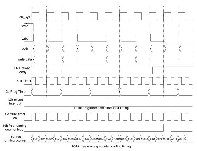
Figure 17-4. 16-bit Free Running Counter Loading Timing Diagram
