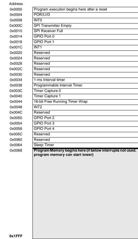
Figure 10-1. Program Memory Space with Interrupt Vector Table
