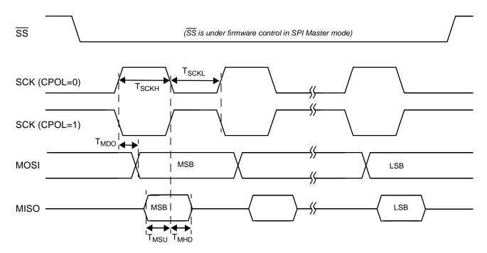
Figure 21-2. SPI Master Timing, CPHA = 1
