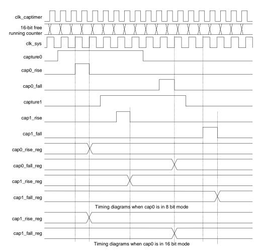
Figure 17-3. Timer Functional Timing Diagram
