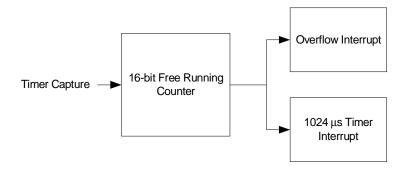
Figure 17-1. 16-bit Free Running Counter Block Diagram
