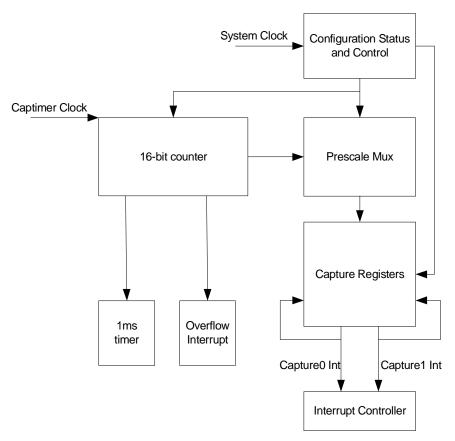
Figure 11-3. Timer Capture Block Diagram
