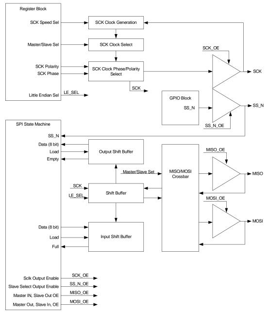
Figure 16-1. SPI Block Diagram
