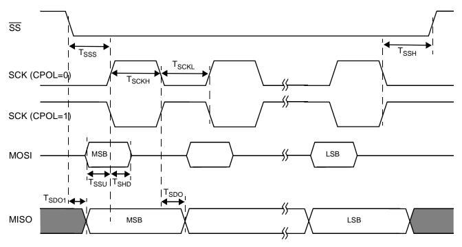
Figure 21-5. SPI Slave Timing, CPHA = 0
