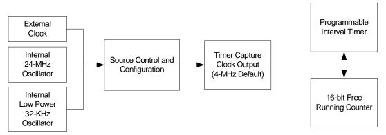
Figure 17-2. Time Capture Block Diagram
