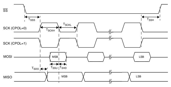
Figure 21-3. SPI Slave Timing, CPHA = 1
