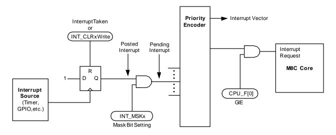
Figure 18-1. Interrupt Controller Block Diagram
