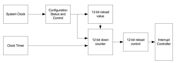
Figure 11-2. Programmable Interval Timer Block Diagram
