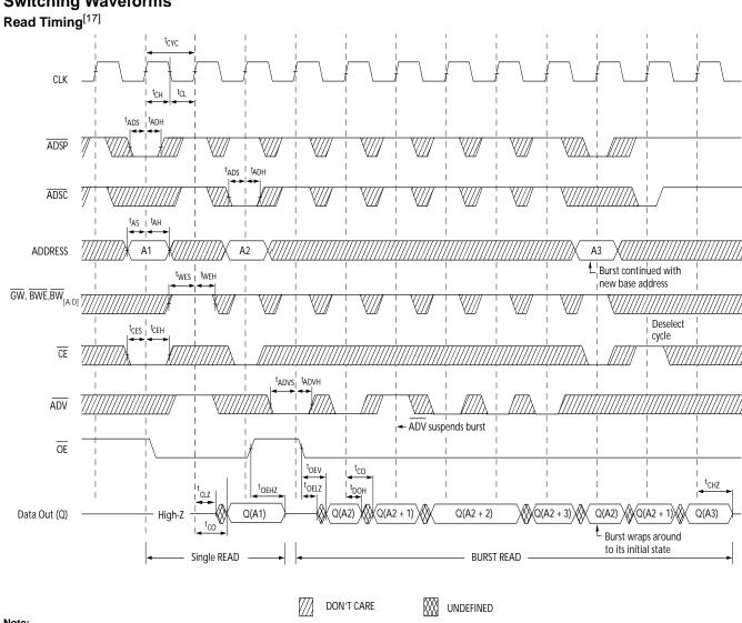
17. On this diagram, when  $\overline{CE}$  is LOW,  $\overline{CE}_1$  is LOW,  $\overline{CE}_2$  is HIGH and  $\overline{CE}_3$  is LOW. When  $\overline{CE}$  is HIGH,  $\overline{CE}_1$  is HIGH or  $\overline{CE}_2$  is LOW or  $\overline{CE}_3$  is HIGH.
