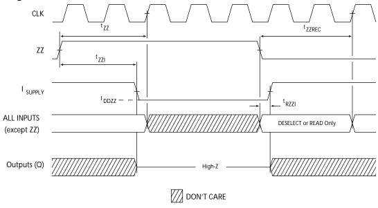
26. Device must be deselected when entering ZZ mode. See Cycle Descriptions table for all possible signal conditions to deselect the device. 27. DQs are in high-Z when exiting ZZ sleep mode.
