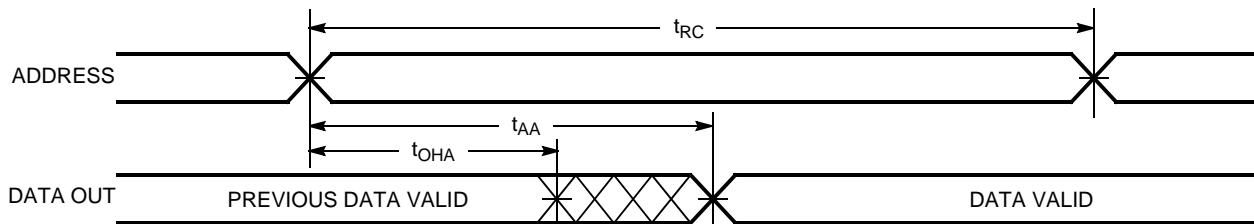
Read Cycle No. 2 ( $\overline{OE}$  Controlled)<sup>[11, 12]</sup>
