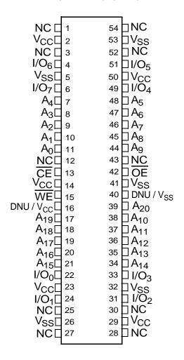
1. DNU / V<sub>CC</sub> Pin (#16) has to be left floating or connected to V<sub>CC</sub> and DNU / V<sub>SS</sub> Pin (#40) has to be left floating or connected to V<sub>SS</sub> to ensure proper application.
