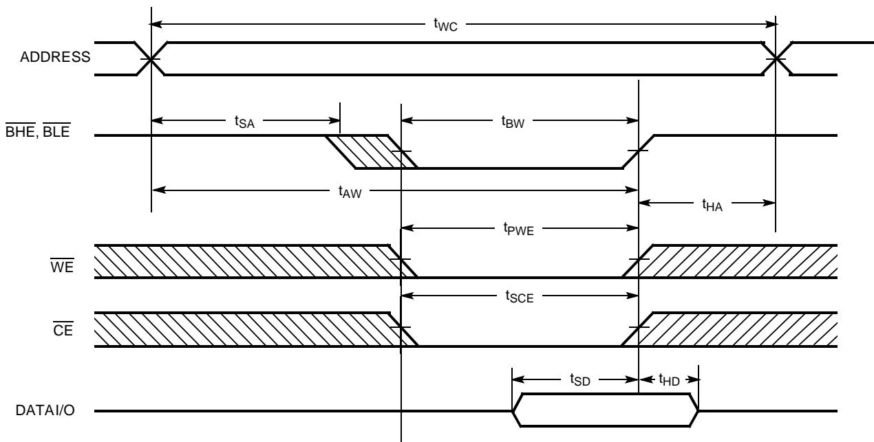
**Write Cycle No. 3 ( $\overline{\text{WE}}$  Controlled,  $\overline{\text{OE}}$  LOW)<sup>[13, 14, 15]</sup>**
