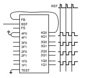
**Figure 4. Inverted Output Connections**
