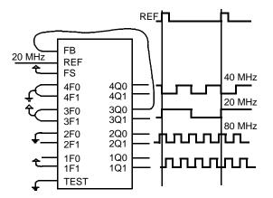
Figure 5. Frequency Multiplier with Skew Connections
