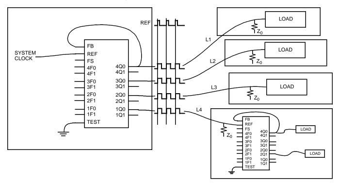
Figure 8. Board-to-Board Clock Distribution
