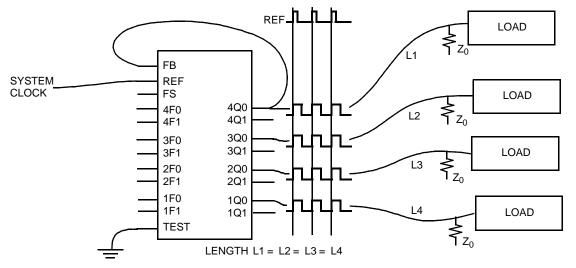
Figure 2. Zero-Skew and/or Zero-Delay Clock Driver
