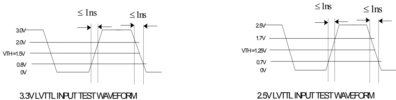
Figure 2. LVTTTL Output Test Waveforms
