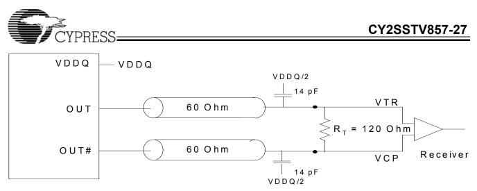
Figure 6. Differential Signal Using Direct Termination Resistor
