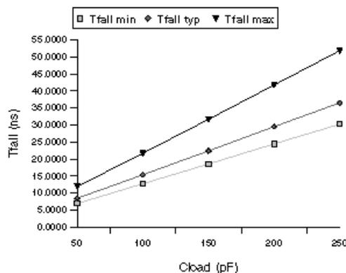
Figure 4. 400 pF Buffer Response (Data from simulation)
