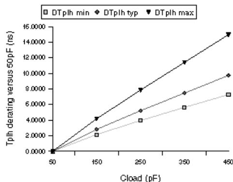
$\Delta T_{phi}$  ( $V_{ref} V_{cc}/2$ )
