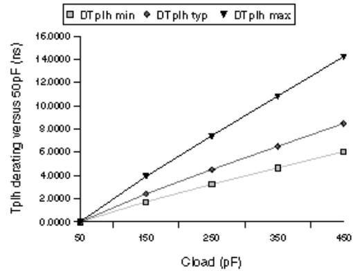
$\Delta T_{phl}$  ( $V_{ref} V_{cc}/2$ )
