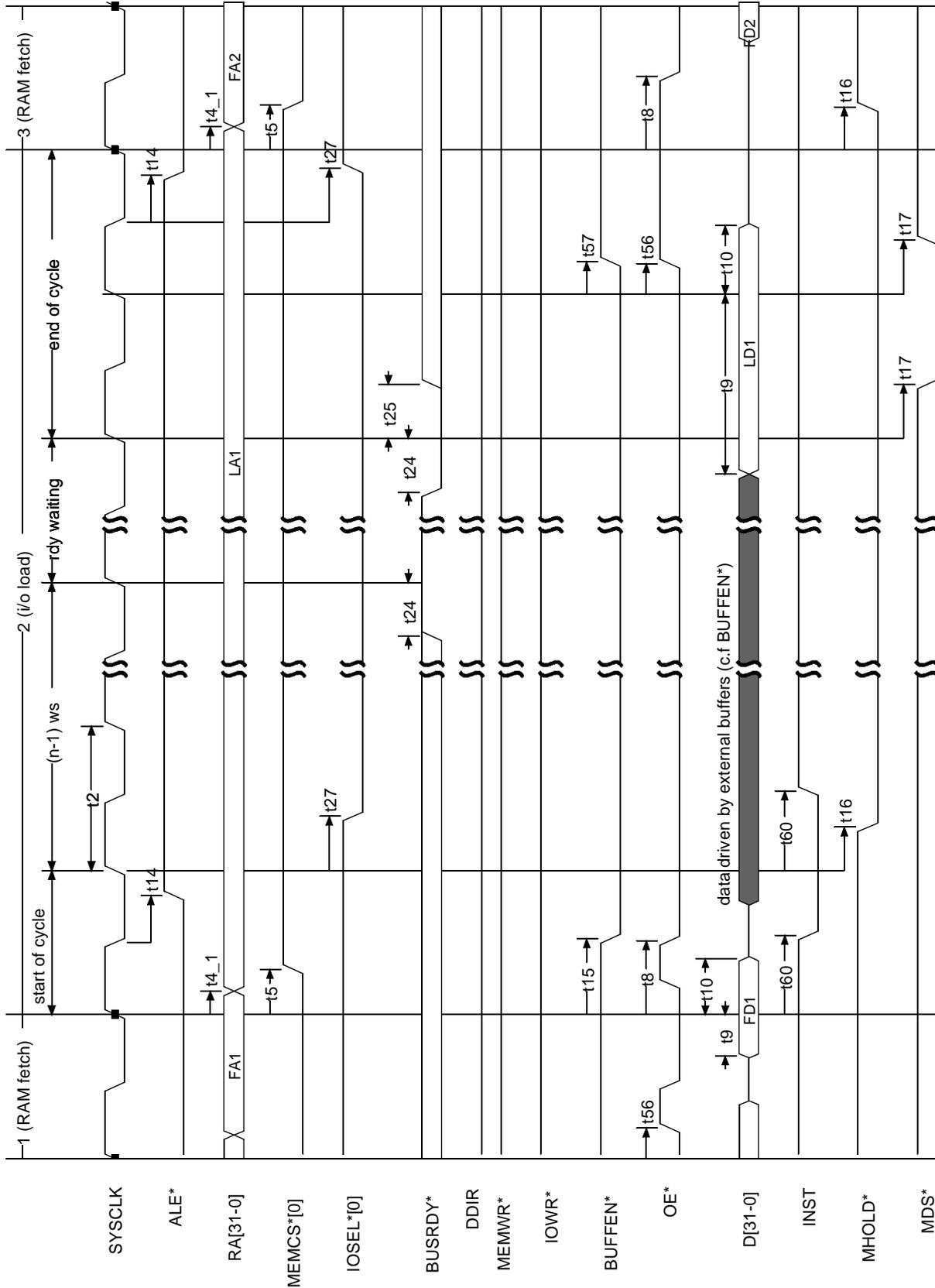
Figure 14. EXCHANGE RAM Store with BUSDRY\* and n Waitstates
