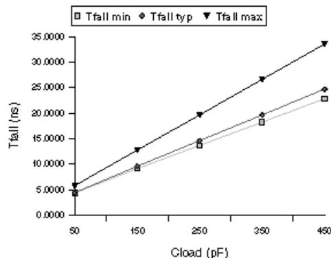
Figure 5. OE\*/400 pF Buffer Response (Data from simulation)
