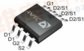
Top View of SOP – 8
