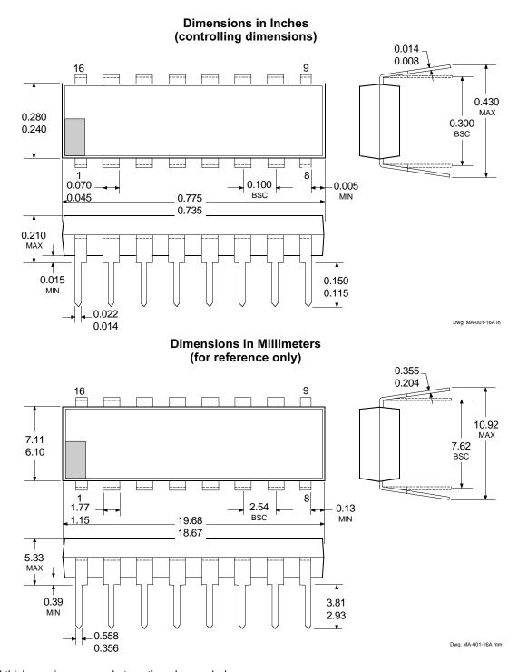
NOTES: 1. Lead thickness is measured at seating plane or below.
