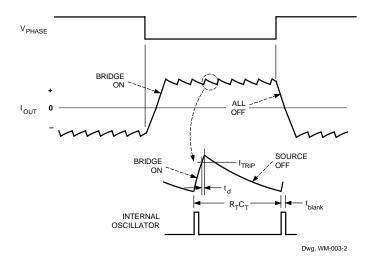
The frequency of the internal clock oscillator is set by the external timing components  $R_TC_T$ . The frequency can be approximately calculated as:
