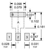
Pads 1, 2, 3, and A — Standard SOT89 Layout Pads 1, 2, 3, and B — Low-Stress Version
