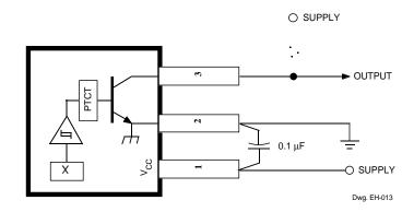
The simplest form of magnet that will operate these devices is a ring magnet. Other methods of operation, such as linear magnets, are possible.
