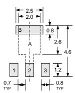
Pads 1, 2, 3, and A — Standard SOT89 Layout Pads 1, 2, 3, and B — Low-Stress Version
