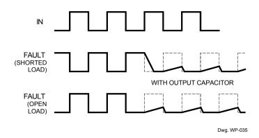
Under some conditions it is possible to get spurious glitches on the FAULT output at load turn-on and turn-off transitions:
