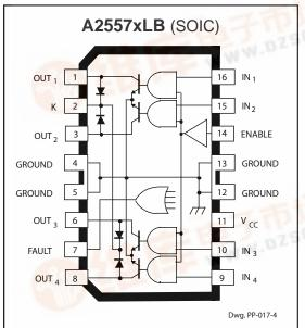
Note that the A2557xB (DIP) and the A2557xLB (SOIC) are electrically identical and share a common terminal number assignment.
