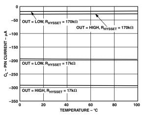
TPC 5. Current Limit Programming Current vs. Temperature
