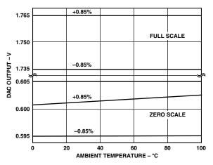
TPC 2. DAC Output Voltage vs. Temperature
