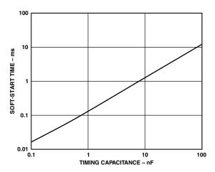
TPC 6. Soft-Start Time vs. Timing Capacitance
