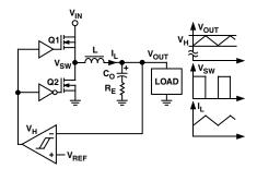
Figure 1. Conventional Hysteretic Regulator and Its Characteristic Waveforms
