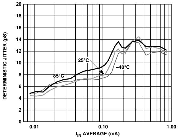
Figure 17. Deterministic Jitter vs. Input Current (K28.5 @ 4.25 Gbps)
