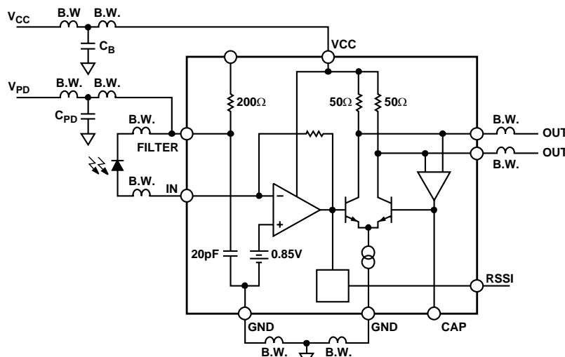
Figure 20. Equivalent Circuit of Assembly Including Bond Wires
