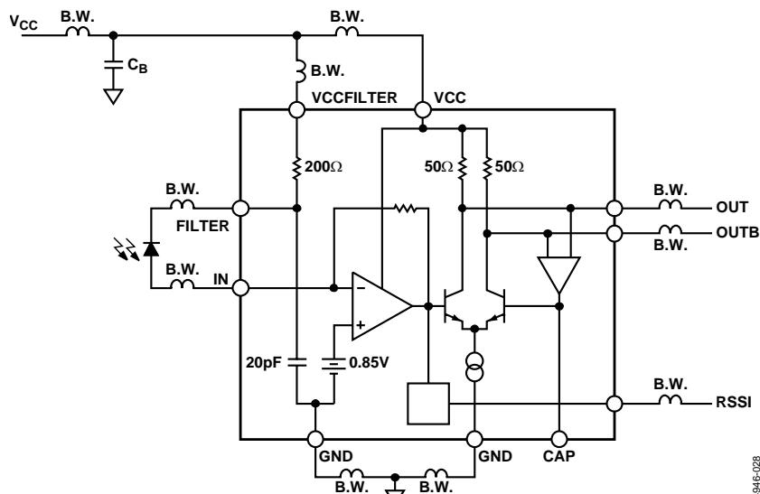
Figure 23. Equivalent Circuit of the Assembly Including Bond Wires
