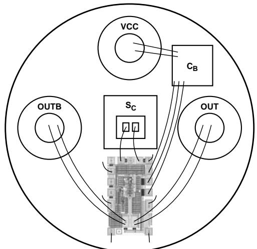
Figure 24. 4-Pin TO-46 with Internal PD Biasing
