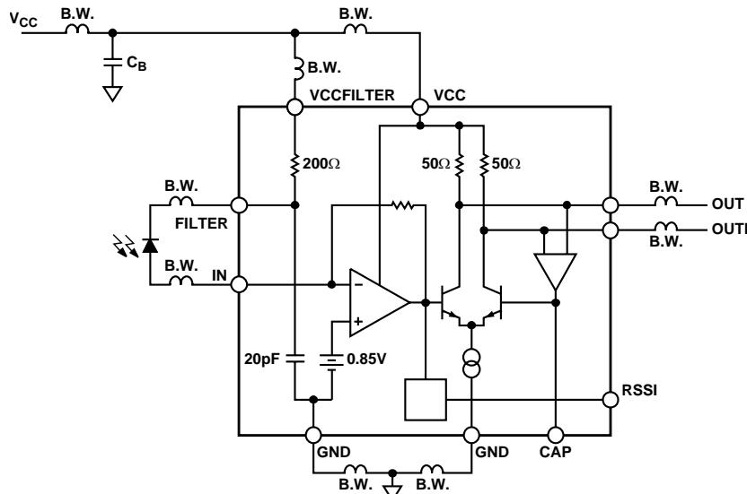
Figure 26. Equivalent Circuit of Assembly Including Bond Wires
