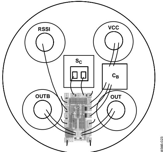
Figure 21. 5-Pin TO-46 with Internal PD Biasing and RSSI Output
