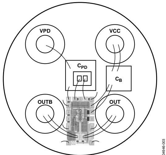
Figure 18. 5-Pin TO-46 with External Photodiode Supply VPD
