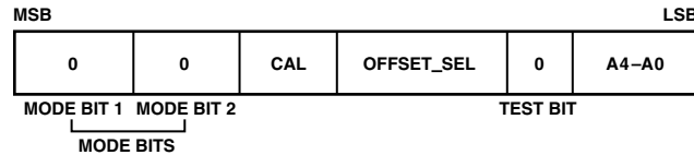
a. 10-Bit Input Serial Write Word (ISHA Mode)
