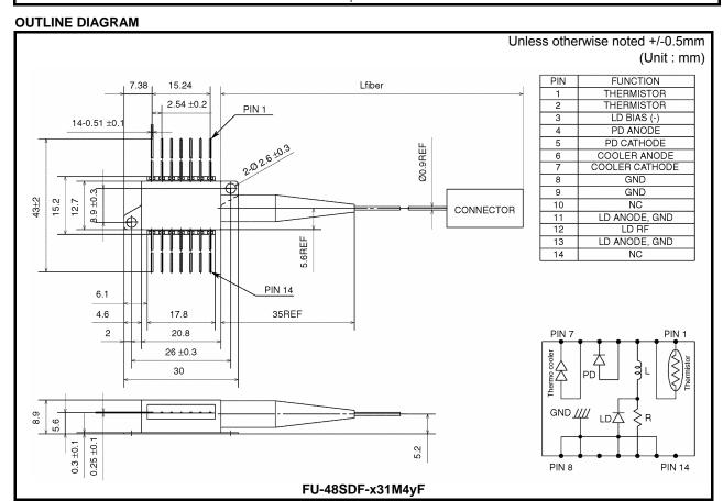
1.3  $\mu\text{m}$  DFB-LD MODULE WITH SINGLEMODE FIBER PIGTAIL
