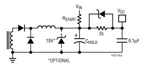
Figure 5a. Auxiliary Winding Bias Supply
