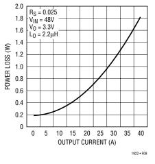
Figure 9. R<sub>SENSE</sub> Power Loss vs I<sub>OUT</sub>
