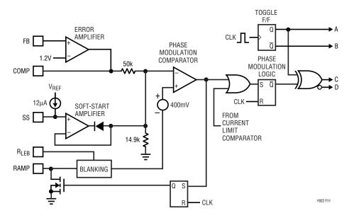
Figure 11. Phase Modulation Circuitry
