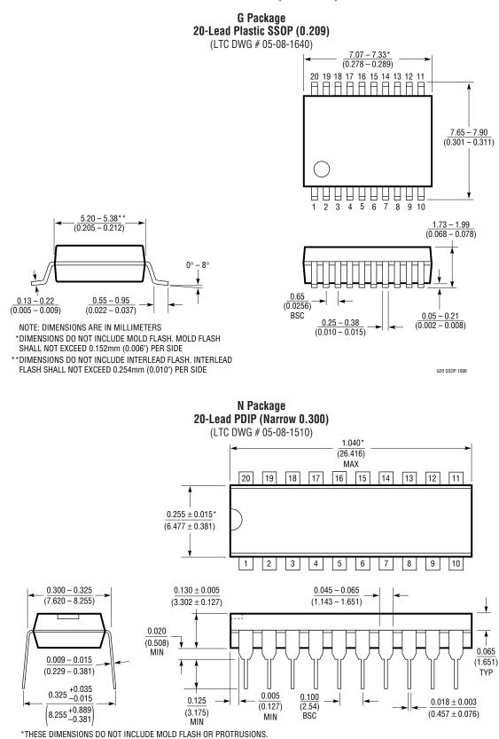
MOLD FLASH OR PROTRUSIONS SHALL NOT EXCEED 0.010 INCH (0.254mm)
