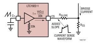
Figure 7. Slope Compensation Circuitry
