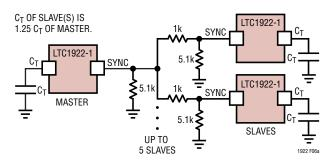
Figure 6a. SYNC Output (Master Mode)
