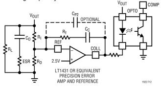
Figure 12. Compensation for Polymer Electrolytic
