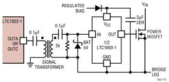
Figure 15. High Side Gate Driver Circuitry
