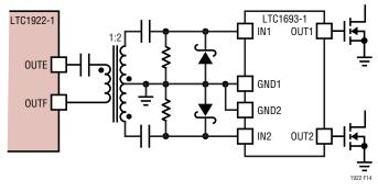
Figure 14. Isolated Drive Circuitry
