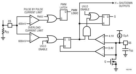
Figure 8. Current Sense/Fault Circuitry Detail
