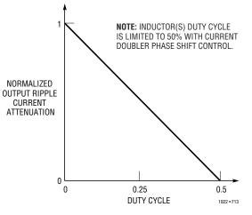
Figure 13. Ripple Current Cancellation vs Duty Cycle
