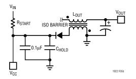
Figure 5b. Output Inductor Bias Supply
