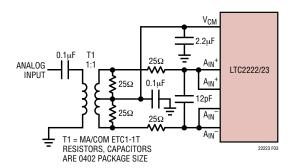
Figure 3. Single-Ended to Differential Conversion
