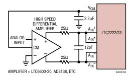
Figure 4. Differential Drive with an Amplifier
