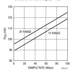
LTC2222:  $IOV_{DD}$  vs Sample Rate, 5MHz Sine Wave Input,  $-1dB, OV_{DD} = 1.8V$
