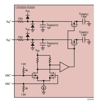
Figure 2. Equivalent Input Circuit
