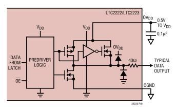
Figure 13. Digital Output Buffer
