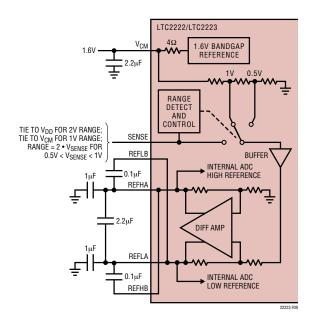
Figure 9. Equivalent Reference Circuit
