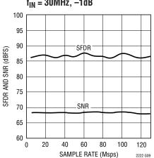
LTC2222: SFDR and SNR vs Sample Rate, 1V Range, f<sub>IN</sub> = 30MHz, -1dB
