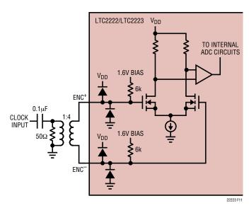
Figure 11. Transformer Driven ENC+/ENC-
