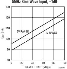
LTC2223: IOV<sub>DD</sub> vs Sample Rate, 5MHz Sine Wave Input, -1dB,OV<sub>DD</sub> = 1.8V
