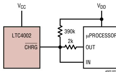
Figure 1. Microprocessor Interface
