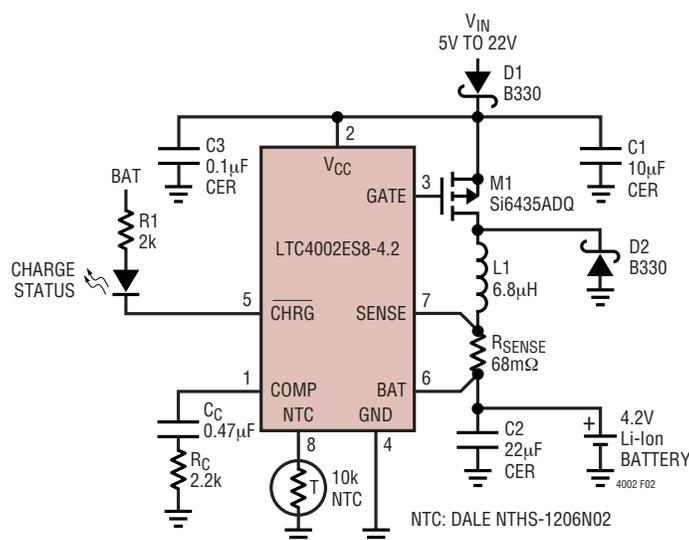
Figure 2. 1.5A Single Cell Li-Ion Battery Charger
