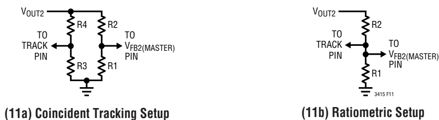
Figure 11. Setup for Tracking and Ratiometric Sequencing
