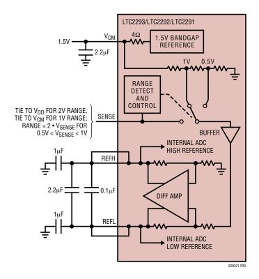
Figure 9. Equivalent Reference Circuit
