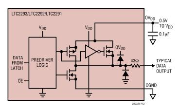
Figure 12. Digital Output Buffer
