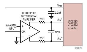
Figure 4. Differential Drive with an Amplifier
