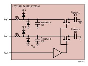
Figure 2. Equivalent Input Circuit
