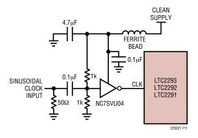
Figure 11. Sinusoidal Single-Ended CLK Drive
