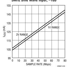
LTC2293:  $I_{OVDD}$  vs Sample Rate, 5MHz Sine Wave Input, -1dB,  $O_{VDD}$  = 1.8V
