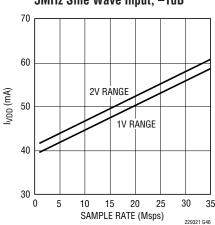
LTC2291: I<sub>OVDD</sub> vs Sample Rate, 5MHz Sine Wave Input, -1dB, 0<sub>VDD</sub> = 1.8V
