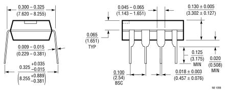
\*THESE DIMENSIONS DO NOT INCLUDE MOLD FLASH OR PROTRUSIONS. MOLD FLASH OR PROTRUSIONS SHALL NOT EXCEED 0.010 INCH (0.254mm)
