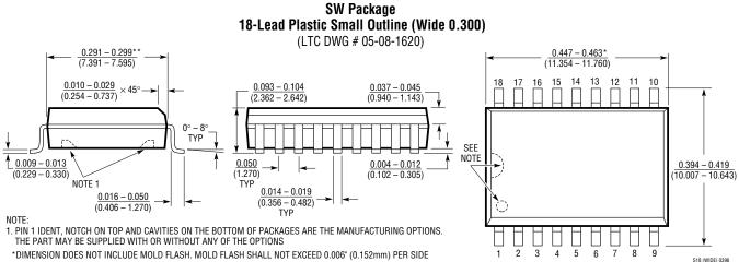
\*\*DIMENSION DOES NOT INCLUDE INTERLEAD FLASH. INTERLEAD FLASH SHALL NOT EXCEED 0.010" (0.254mm) PER SIDE
