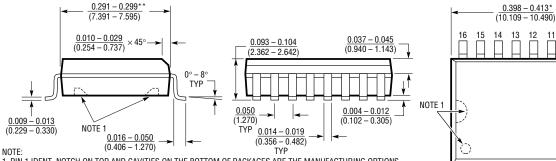
1. PIN 1 IDENT, NOTCH ON TOP AND CAVITIES ON THE BOTTOM OF PACKAGES ARE THE MANUFACTURING OPTIONS. THE PART MAY BE SUPPLIED WITH OR WITHOUT ANY OF THE OPTIONS
