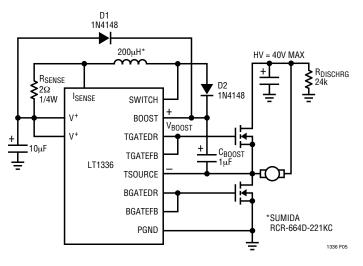
Figure 5. Driving a Supply Referenced Motor
