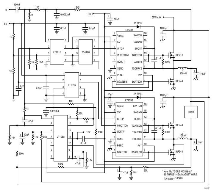
Figure 7. 200W Class D, 10Hz to 1kHz Amplifier
