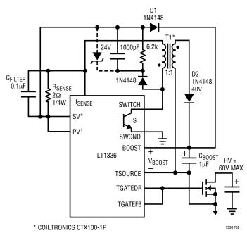
Figure 2. Using the Flyback Regulator
