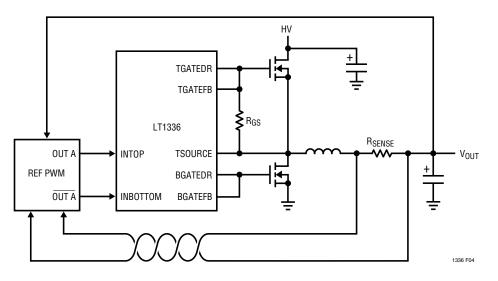
Figure 4. Adding Synchronous Switching to a Step-Down Switching Regulator
