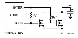
Figure 3. Paralleling MOSFETs
