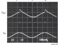
Figure 2. Lowpass Slope Limiting Filter with 0 TC
