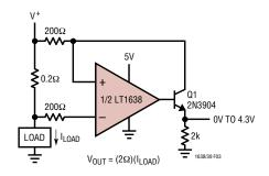
Figure 3. Positive Supply Rail Current Sense
