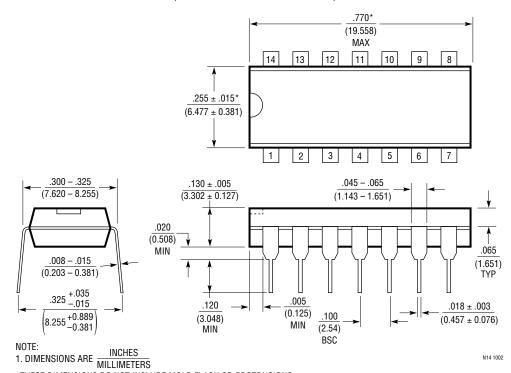
\*THESE DIMENSIONS DO NOT INCLUDE MOLD FLASH OR PROTRUSIONS. MOLD FLASH OR PROTRUSIONS SHALL NOT EXCEED .010 INCH (0.254mm)
