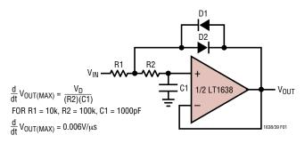
Figure 1. Lowpass Slope Limiting Filter
