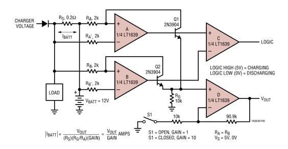
Figure 5. Battery Monitor
