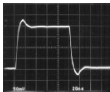
Small-Signal Transient (AV = -1)
