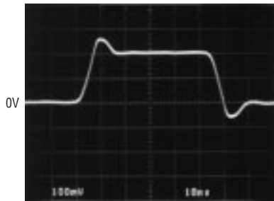
5V Small-Signal Response
