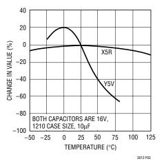
Figure 3. Ceramic Capacitor Temperature Characterics
