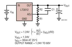
Figure 1. Adjustable Operation
