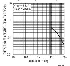
10Hz to 100kHz Output Noise
