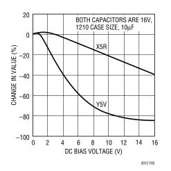
Figure 2. Ceramic Capacitor DC Bias Characterics
