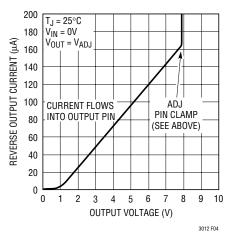
Figure 4. Reverse Output Current
