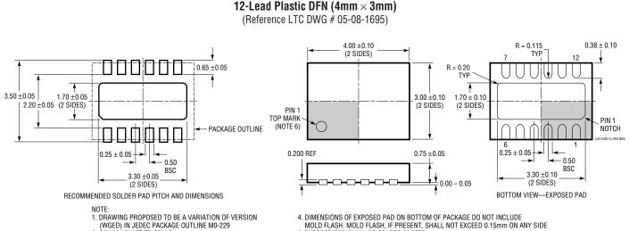
DE Package 12-Lead Plastic DFN (4mm  $\times$  3mm)
