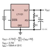
Figure 1. Adjustable Operation
