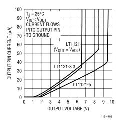
Figure 2. Reverse Output Current
