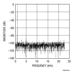
Figure 16a. LTC1294 FFT Plot  $f_{IN} = 1 kHz$ ,  $f_S = 45.4 kHz$ , SNR = 72.7dB with  $\pm 5 V$  Supplies
