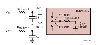
Figure 7. Analog Input Equivalent Circuit
