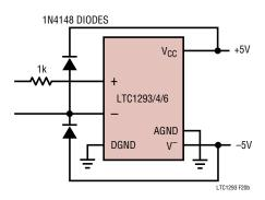
Figure 20b. Overvoltage Protection for Inputs
