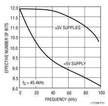
Figure 17. LTC1294 ENOB vs Input Frequency
