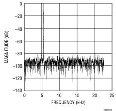
Figure 18. LTC1294 FFT Plot  $f_{\text{IN}}1$  = 5.1kHz,  $f_{\text{IN}}2$  = 5.6kHz,  $f_{\text{S}}$  = 45.4kHz with  $\pm$ 5V Supplies
