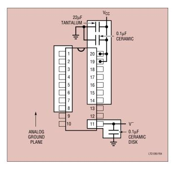
Figure 4. Ground Plane for the LTC1293/4/6
