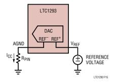
Figure 15. Parasitic Pin Resistance (R<sub>PIN</sub>)
