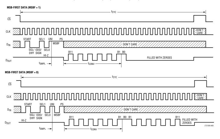
Power Shutdown Operating Sequence Example: Differential Inputs (CH4<sup>+</sup>, CH5<sup>-</sup>), Unipolar Mode and MSB-First Data
