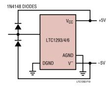
Figure 19. Overvoltage Protection for Inputs
