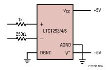
Figure 20a. Overvoltage Protection for Inputs
