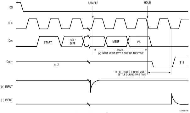
Figure 8. "+" and "-" Input Settling Windows
