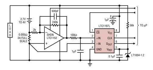
Figure 14. This OA to 2A Battery Current Monitor Draws Only  $45\mu A$  from a 3V Battery
