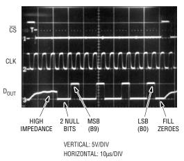
Figure 12. Scope Photo of the LTC1197 "Quick Look" Circuit Waveforms Showing A/D Output 1001001001 (249<sub>HEX</sub>)
