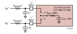
Figure 6. Analog Equivalent Circuit
