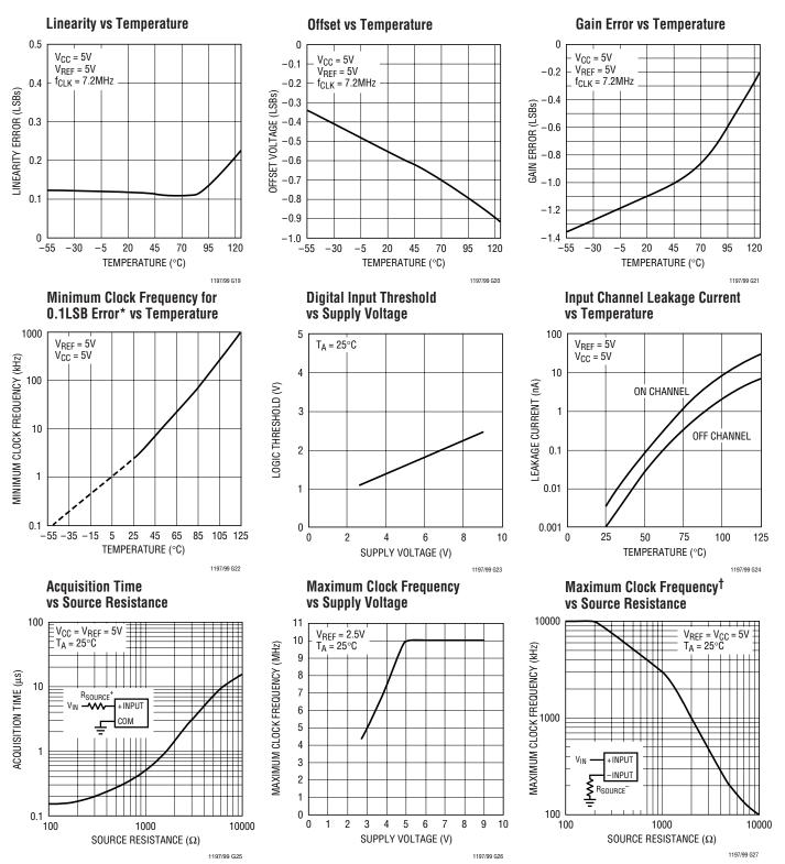
\* As the CLK frequency is decreased from 2MHz, minimum CLK frequency ( $\Delta$ error  $\leq$  0.1LSB) represents the frequency at which a 0.1LSB shift in any code translation from its 2MHz value is first detected.
