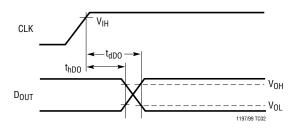
Voltage Waveforms for t<sub>dis</sub>
