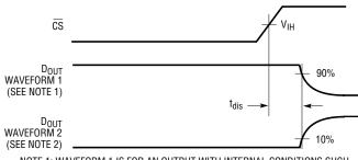
NOTE 1: WAVEFORM 1 IS FOR AN OUTPUT WITH INTERNAL CONDITIONS SUCH THAT THE OUTPUT IS HIGH UNLESS DISABLED BY THE OUTPUT CONTROL NOTE 2: WAVEFORM 2 IS FOR AN OUTPUT WITH INTERNAL CONDITIONS SUCH THAT THE OUTPUT IS LOW UNLESS DISABLED BY THE OUTPUT CONTROL 1197/99 TCOS
