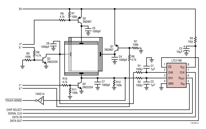
Figure 13. The LTC1199 Digitizes Resistive Touchscreen X and Y Axis Voltages. The ADC's Auto Shutdown Feature Helps Maximize Battery Life in Portable Touchscreen Equipment
