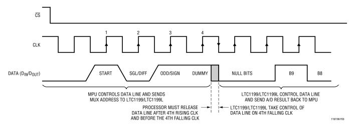
Figure 3. LTC1199/LTC1199L Operation with  $D_{IN}$  and  $D_{OUT}$  Tied Together
