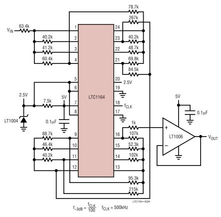
Figure 12. 8th Order Lowpass Single Supply Elliptic-Bessel Transitional Filter Total Supply Current = 4mA, Passband Noise  $50\mu V_{RMS}$
