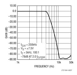
Figure 14. LTC1164 8th Order Lowpass Elliptic, f<sub>CUTOFF</sub> = 5kHz
