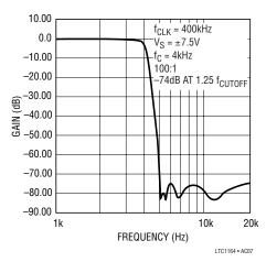
Figure 16. LTC1164 9th Order Lowpass Elliptic, f<sub>CUTOFF</sub> = 4kHz
