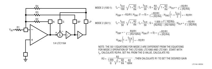
Figure 9. Mode 2: 2nd Order Filter Providing Notch, Bandpass, Lowpass
