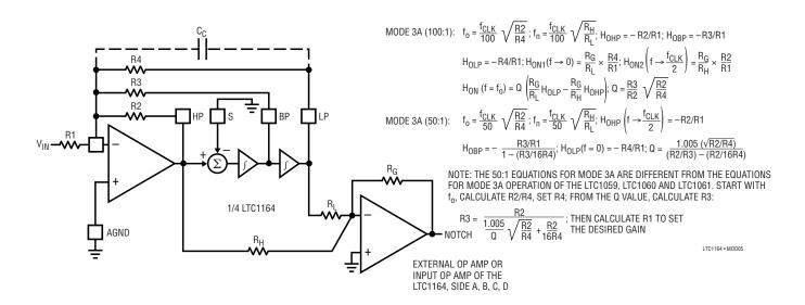
Figure 10. Mode 3A: 2nd Order Filter Providing Highpass, Bandpass, Lowpass, Notch
