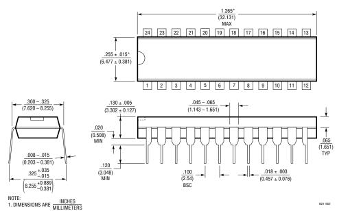
\*THESE DIMENSIONS DO NOT INCLUDE MOLD FLASH OR PROTRUSIONS. MOLD FLASH OR PROTRUSIONS SHALL NOT EXCEED .010 INCH (0.254mm)
