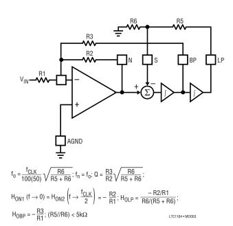
Figure 8. Mode 1b: 2nd Order Filter Providing Notch, Bandpass, Lowpass
