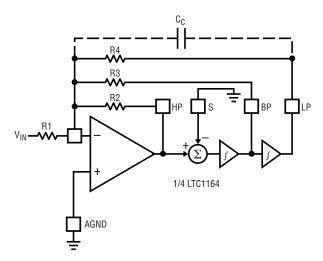
$$\begin{split} \text{MODE 3 (100:1):} \qquad & f_0 = \frac{f_{CLK}}{100} \ \sqrt{\frac{R2}{R4}}; \ Q = \frac{R3}{R2} \ \sqrt{\frac{R2}{R4}}; \ H_{OHP} = - \ R2/R1; \\ H_{OBP} = - \ R3/R1; \ H_{OLP} = - \ R4/R1 \end{split}$$
