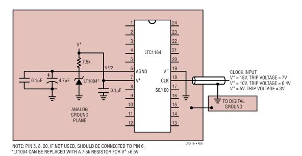
Figure 2. Single Supply Operation
