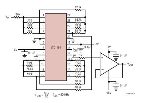
Figure 11. 8th Order Lowpass Butterworth, Passband Noise  $90\mu V_{RMS}$  (Also Refer to the LTC1164-5)
