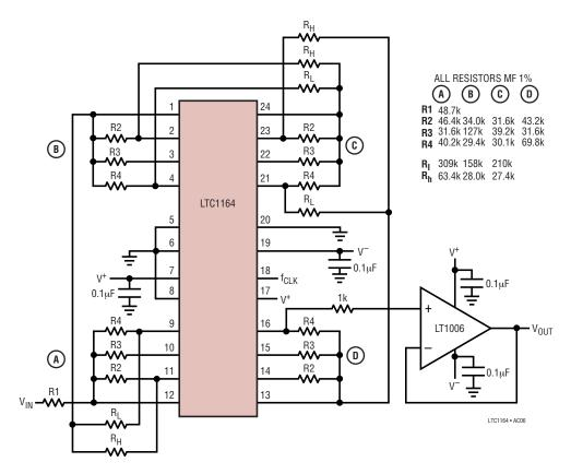
Figure 13. LTC1164 8th Order Lowpass Elliptic,  $f_{CUTOFF}$  = 5kHz,  $f_{CLK}$  = 250kHz, -78dB at 10kHz, Passband Noise = 110 $\mu$ V<sub>RMS</sub>  $\pm$ 5V (Also Refer to the LTC1164-6)
