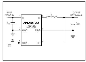
Figure 3. MAX1921 Application Circuit Using Tantalum Output Capacitor
