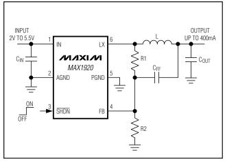
Figure 2. Typical Application Circuit (MAX1920)
