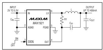
Figure 1. Typical Output Application Circuit (MAX1921)
