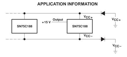
NOTE A: External diodes placed in series with the V<sub>CC+</sub> and V<sub>CC</sub>-leads protect the SN75C188 in the fault condition where the device outputs are shorted to  $\pm$ 15 V and the power supplies are at low voltage and provide low-impedance paths to GND.
