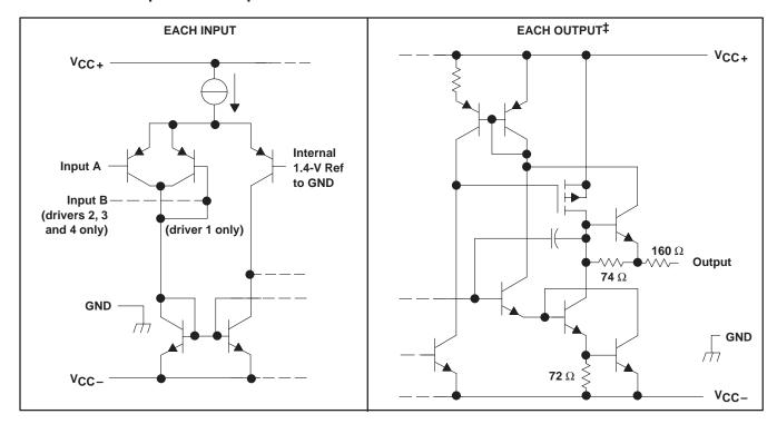
schematics of inputs and outputs
