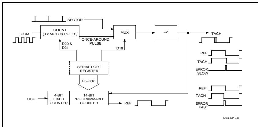
$$\frac{\text{desired}}{\text{total count}} = \frac{60 \times f_{osc}}{\text{desired motor speed (rpm)}}$$
