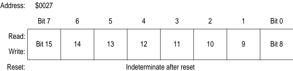
Figure 11-14. TIMA Channel 0 Register High (TACH0H)
