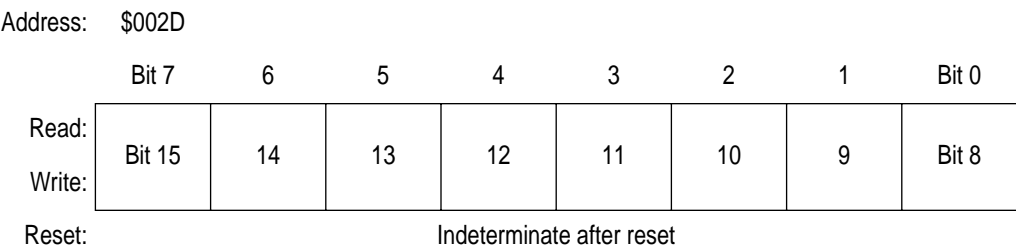
Figure 11-18. TIMA Channel 2 Register High (TACH2H)
