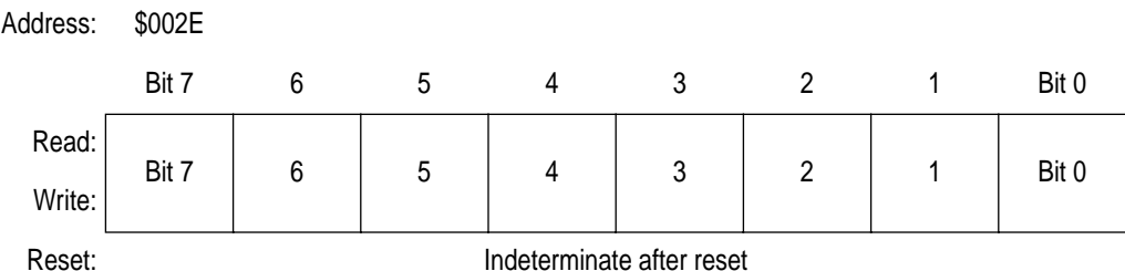
Figure 11-19. TIMA Channel 2 Register Low (TACH2L)
