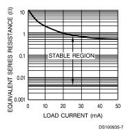
**Important:** The output capacitor must maintain its ESR within the stable region over the full operating temperature range of the application to assure stability.
