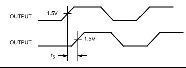
Notes:4. All parameters specified with loaded outputs.5. Duty cycle of input clock is 50%. Rising and falling edge rate is greater than 1 V/ns.
