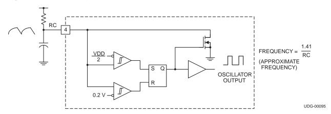
Figure 1. Block Diagram for Oscillator
