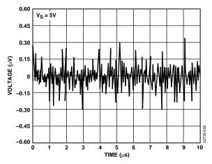
Figure 37. 0.1 Hz to 10 Hz Noise at 5 V
