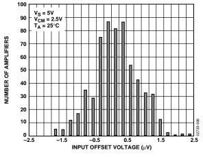
Figure 8. Input Offset Voltage Distribution at 5 V
