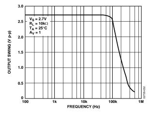
Figure 34. Maximum Output Swing vs. Frequency
