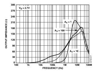
Figure 19. Output Impedance vs. Frequency at 2.7 V
