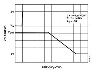
Figure 61. Negative Input Overload Recovery for LMC2001
