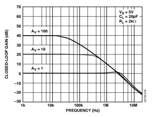
Figure 18. Closed-Loop Gain vs. Frequency at 5 V
