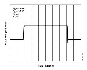
Figure 24. Small Signal Transient Response at 5 V
