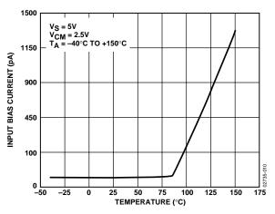
Figure 12. Input Bias Current vs. Temperature
