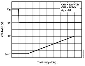
Figure 58. Positive Input Overload Recovery for LMC2001
