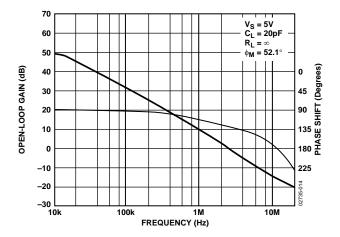
Figure 16. Open-Loop Gain and Phase vs. Frequency
