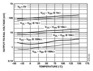
Figure 46. Output-to-Rail Voltage vs. Temperature
