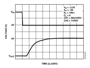
Figure 27. Positive Overvoltage Recovery
