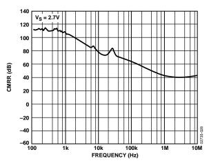
Figure 30. CMRR vs. Frequency at 2.7 V
