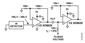
Figure 62. AD8629 Used as Preamplifier for Thermopile
