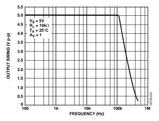
Figure 35. Maximum Output Swing vs. Frequency at 5 V
