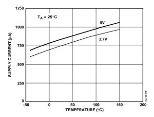
Figure 13. Supply Current vs. Temperature
