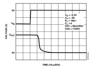
Figure 28. Negative Overvoltage Recovery
