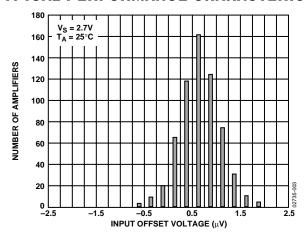
Figure 5. Input Offset Voltage Distribution at 2.7 V
