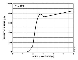
Figure 14. Supply Current vs. Supply Voltage
