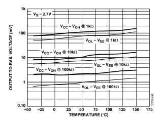
Figure 47. Output-to-Rail Voltage vs. Temperature
