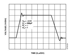
Figure 22. Large Signal Transient Response at 5 V
