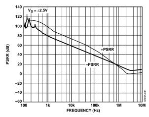
Figure 33. PSRR vs. Frequency
