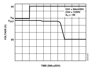
Figure 60. Negative Input Overload Recovery for LTC2050
