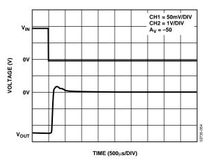
Figure 57. Positive Input Overload Recovery for LTC2050
