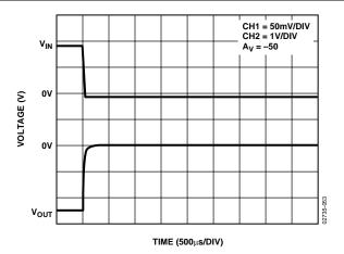
Figure 56. Positive Input Overload Recovery for the AD8628
