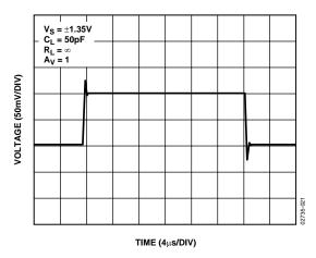
Figure 23. Small Signal Transient Response at 2.7 V
