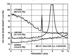
Figure 49. Noise Spectral Density of AD8628 vs. Competition
