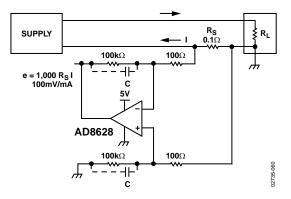
Figure 63. Low-Side Current Sensing
