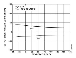
Figure 44. Output Short-Circuit Current vs. Temperature
