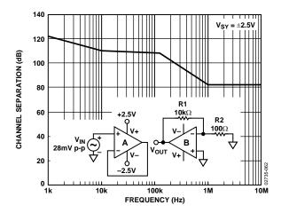
Figure 48. AD8629 Channel Separation
