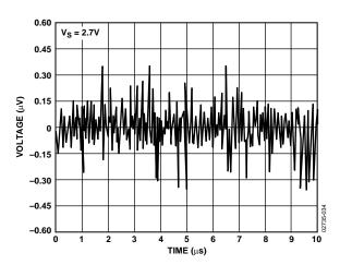
Figure 36. 0.1 Hz to 10 Hz Noise at 2.7 V
