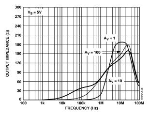
Figure 20. Output Impedance vs. Frequency at 5 V
