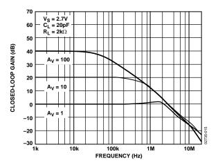
Figure 17. Closed-Loop Gain vs. Frequency at 2.7 V
