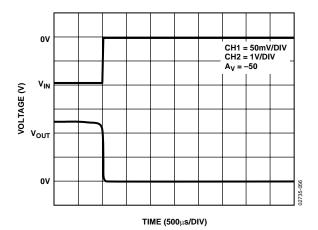
Figure 59. Negative Input Overload Recovery for the AD8628
