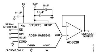
Figure 64. AD8628 Used as an Output Amplifier
