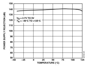
Figure 43. Power Supply Rejection vs. Temperature
