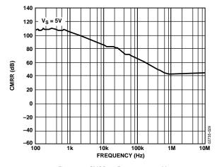
Figure 31. CMRR vs. Frequency at 5  $\rm V$
