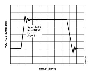
Figure 21. Large Signal Transient Response at 2.7 V
