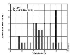
Figure 9. Input Offset Voltage Drift
