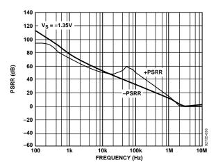
Figure 32. PSRR vs. Frequency
