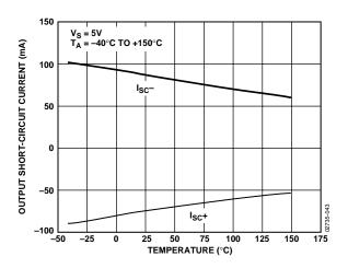
Figure 45. Output Short-Circuit Current vs. Temperature
