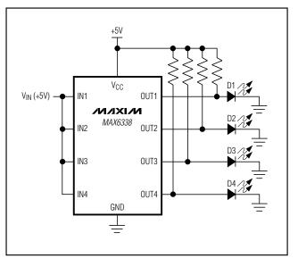
Figure 3. V<sub>CC</sub> Bar Graph Monitoring
