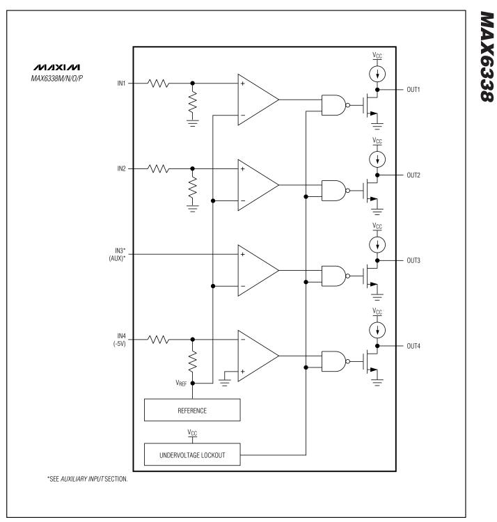
Figure 1. MAX6338 Functional Diagram
