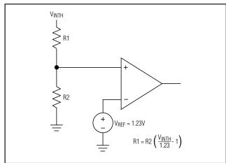
Figure 6. Setting the Auxiliary Monitor
