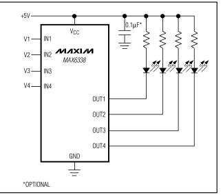
Figure 2. Quad Undervoltage Detector with LED Indicators
