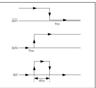
Figure 5. Output Response of Window Detector Circuit
